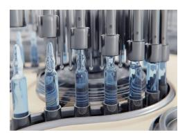
Pharmaceutical manufacturers continue to look to automation for efficient fill/finish of parenteral drugs, and new robotic automation technologies offer the opportunity to further improve flexibility and efficiency. New robotic technologies also aim to eliminate the need to open an isolator to perform interventions to better comply with the European requirements for closed systems.
